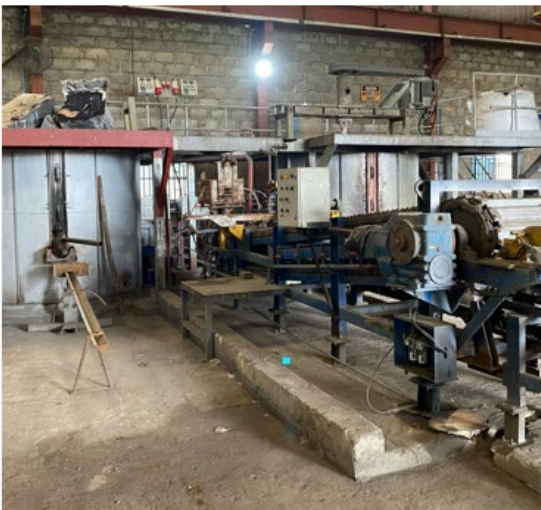
Refining kettles with automated casting machine
