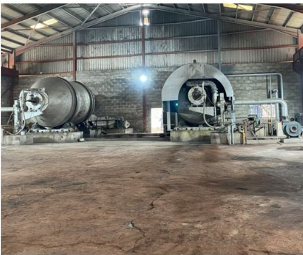
Main smelting hall with the two installed rotary furnaces
