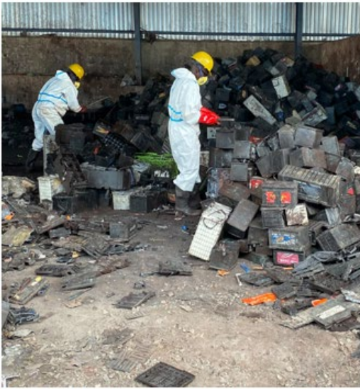
Manual battery breaking with new (unused) PPE
