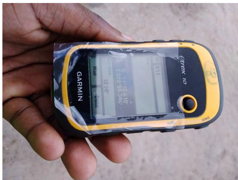
Figure 8: Capturing GPS coordinates on the Garmin Etrex10
