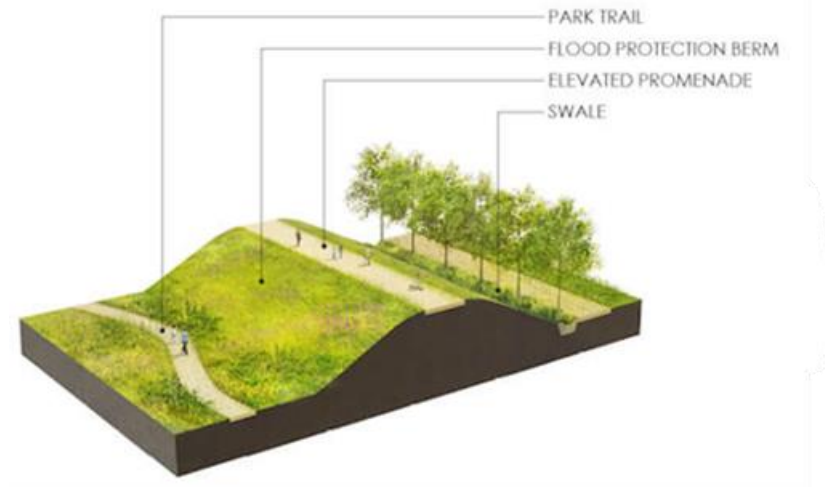
Part E Chapter 4 Figure 12. Illustration of Pedestrian Pathways on a berm (Tzifa, A., & Nikolaidou, S. 2020).
