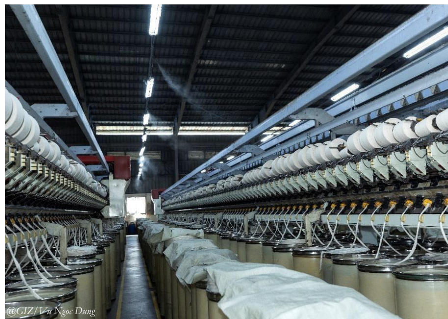
Figure 11 - Spinning yarn from recycled fibres at Tan Nam Trung's factory
