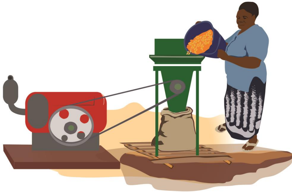
Figure 43 – Milling of orange maize into mealie meal using a hammer mill.
