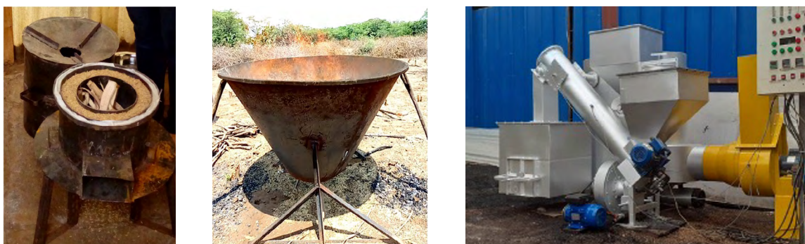
Figure 14: Biochar production systems: top left – cookstove, top right – artisanal kiln, and bottom – air dryer system (Credit: IITA & partners)
