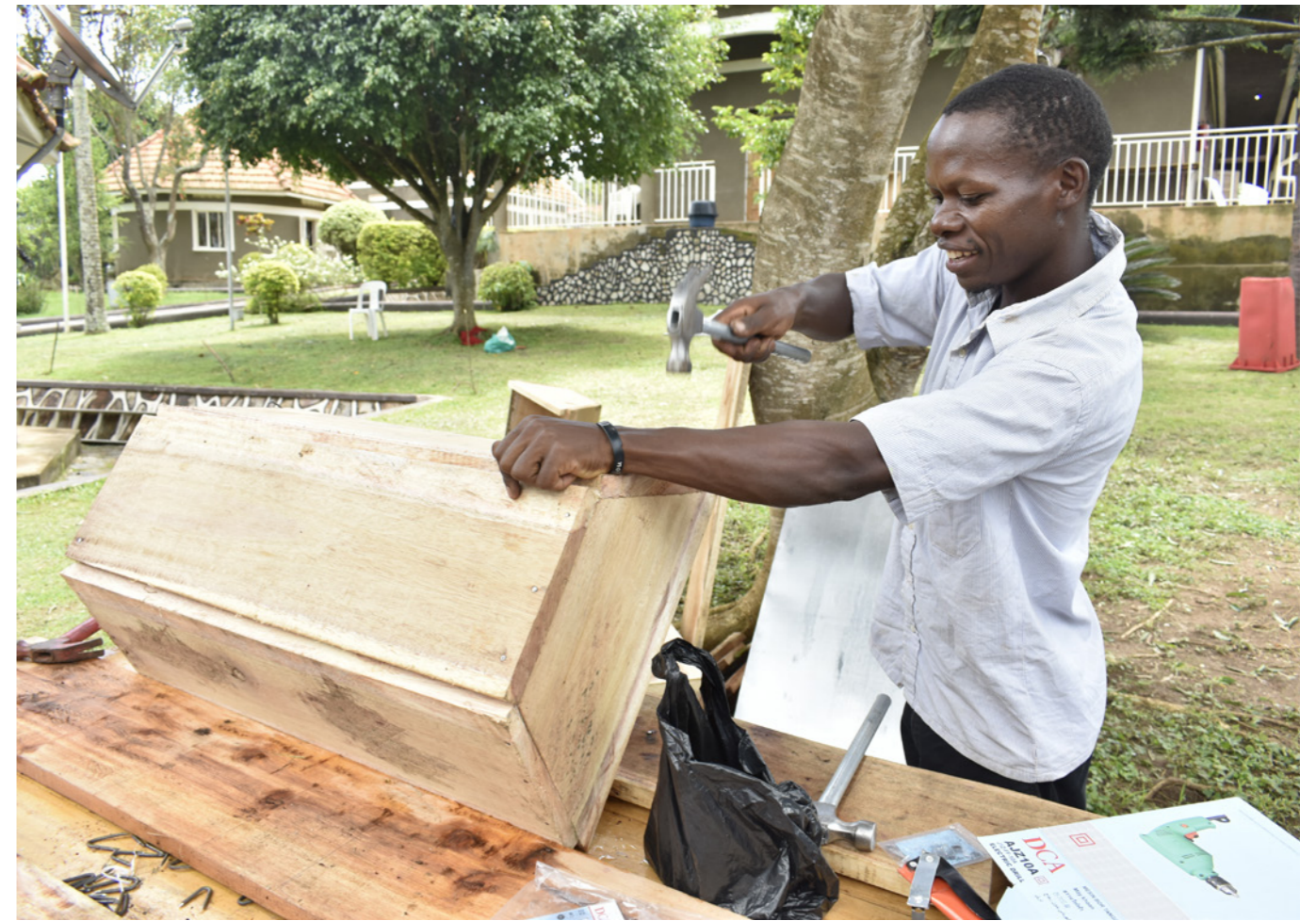
Waswa constructs a Kenya top-bar beehive, at the SSF-U office in Lyantonde. © Jackson Mpagi / SSF-U
