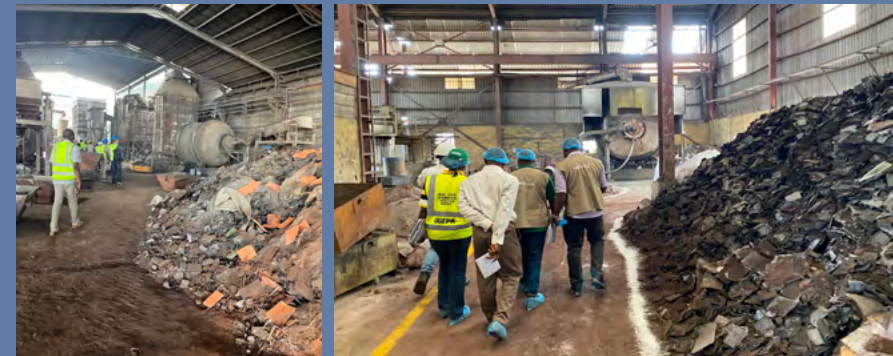
(Left) Poor standards in ULAB recycling companies: Toxic lead dust, unpaved floor, no exhaust system, no occupational safety (Right) Employees of the Nigerian Environmental Protection Agency visit a recycling company
