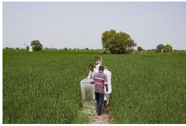
Static gas chamber for GHG sampling: Rice fields in Haryana ©Olam Agri
