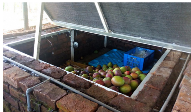
Picture 6. Evaporative cooling chamber (ECC). J-WAFS Abdul Latif Jameel Water & Food Systems La
