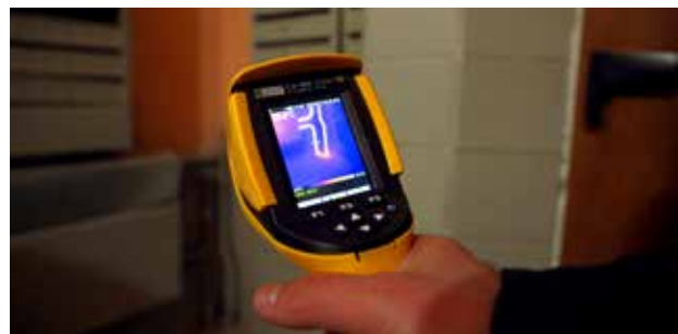
An energy auditor uses a thermal camera to check heat losses in a building.
